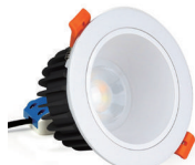
FUT071 12W Beam Angle: 60° Hole Size: ø95-100mm Deep Anti-glare shielding angle >30°
