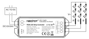
Controller connect to RGB LED strip diagram
