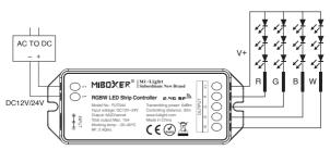
Controller connect to RGBW LED strip diagram
