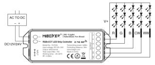
Controller connect to RGB+CCT LED strip diagram
